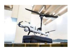
requirement profile for aerial reconnaissance. It flies without almost any noise emission and delivers high-resolution video images from the air via an encrypted data link, contributing to an accurate situational awareness. The Vector longrange reconnaissance drone also is equipped with state-of-the-art digital connectivity to communicate in real time with other systems and achieve an increased combat performance for the whole network.
